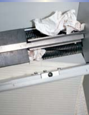
Automatic mechanical feeding system with revolving flaps
