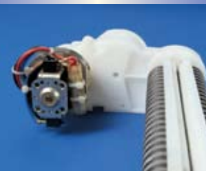
An enclosed transmission system protects the gear from dust and does not require lubrication or maintenance (Kobra S-50)
